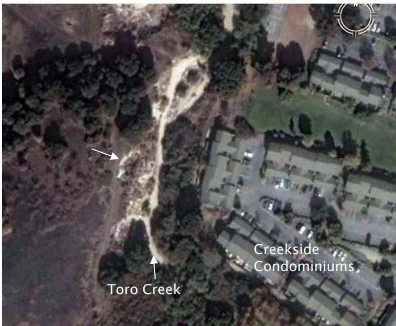
Figure 2: Creekside landslide. Arrow shows headwall scarp.
