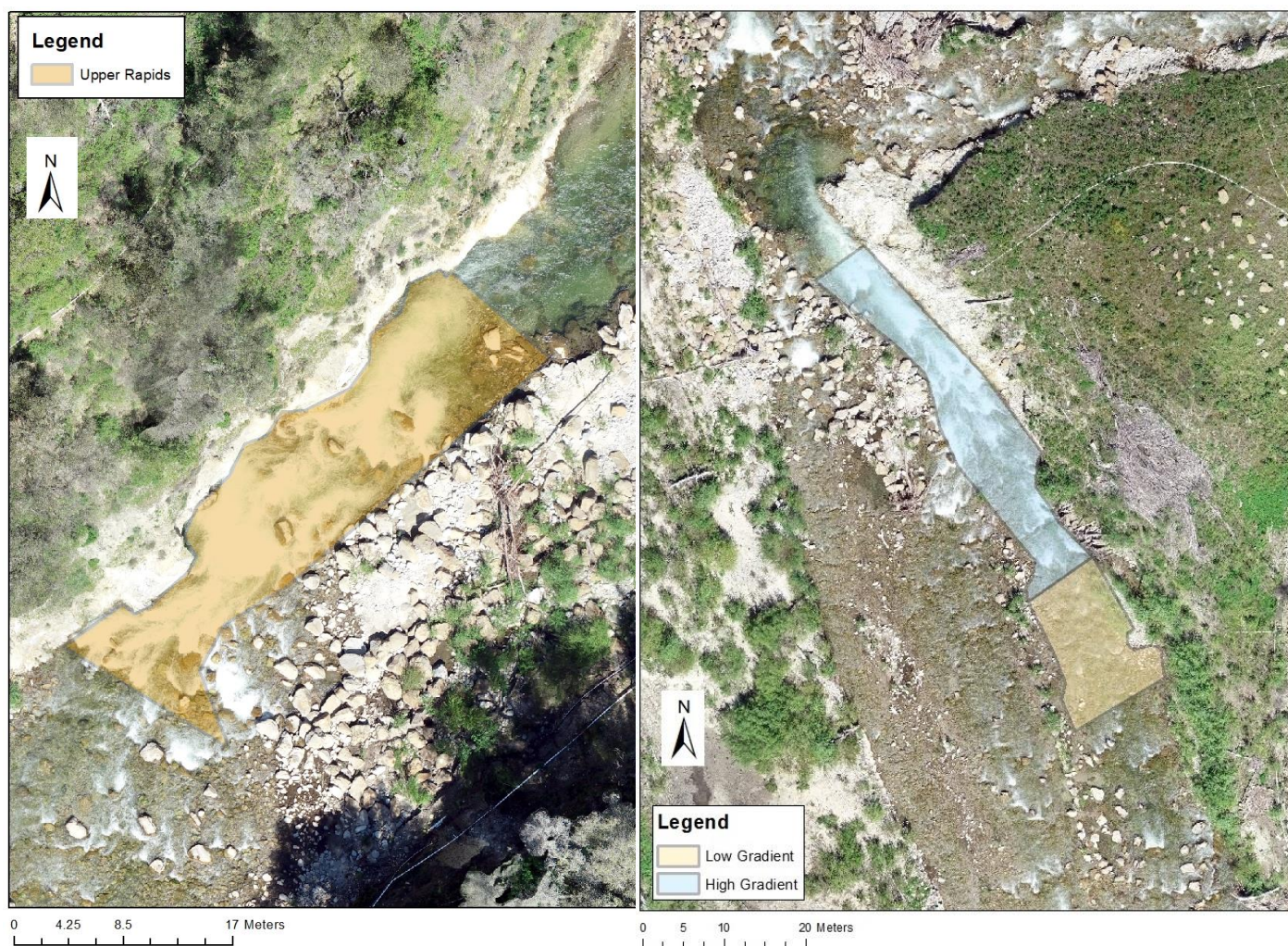
Figure 6. Upper rapids (left), above lower rapids and lower rapids (right) where floats were deployed and sUAS video was taken to estimate surface velocity.
