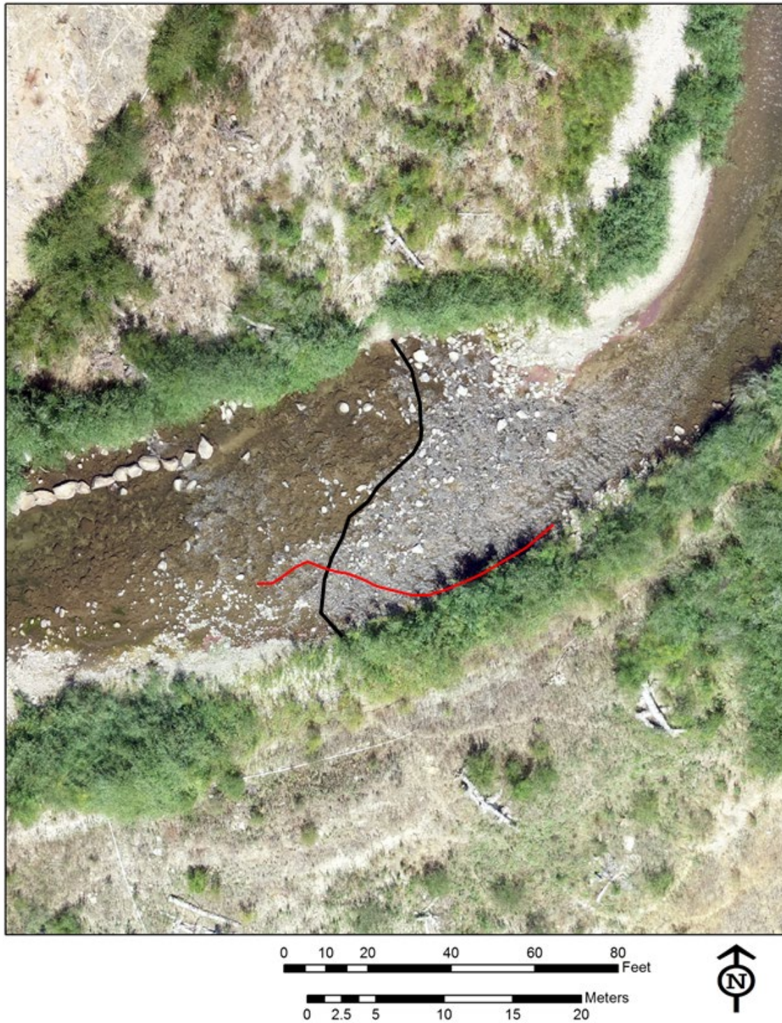
Figure 6: Site 3 with approximate locations of longitudinal profile (red) and cross section (black). Flow is toward the northwest. Background image is orthophoto obtained 8/31/2019 at a flow of 17 cfs.
