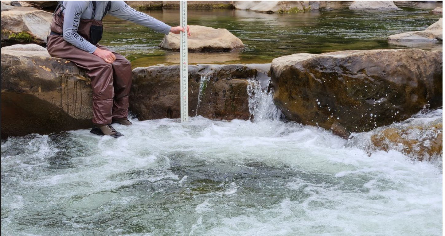
Figure 3. Estimating jump heights and water depths at 70 cfs (May 30, 2023).
