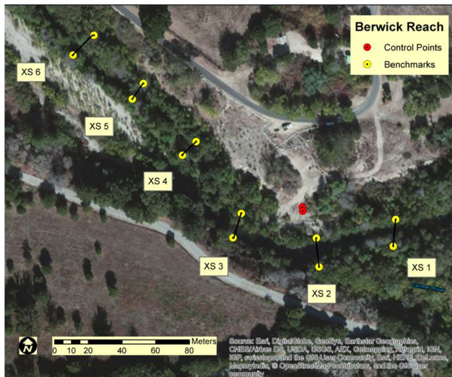
Figure 8. Location of georeferenced control points and cross sections within the Berwick Reach.
