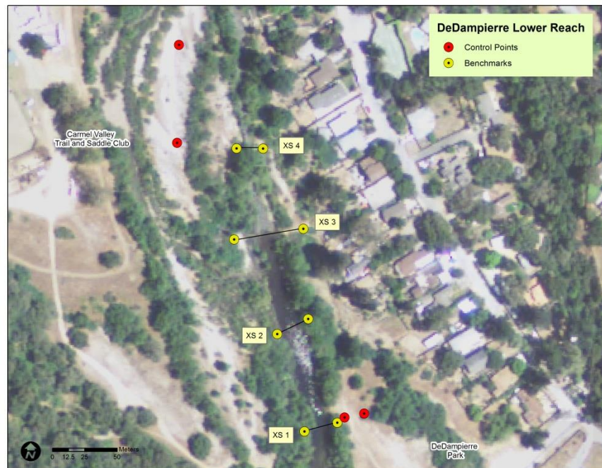
Figure 6. Location of georeferenced control points and cross sections within the DeDampierre Lower Reach.
