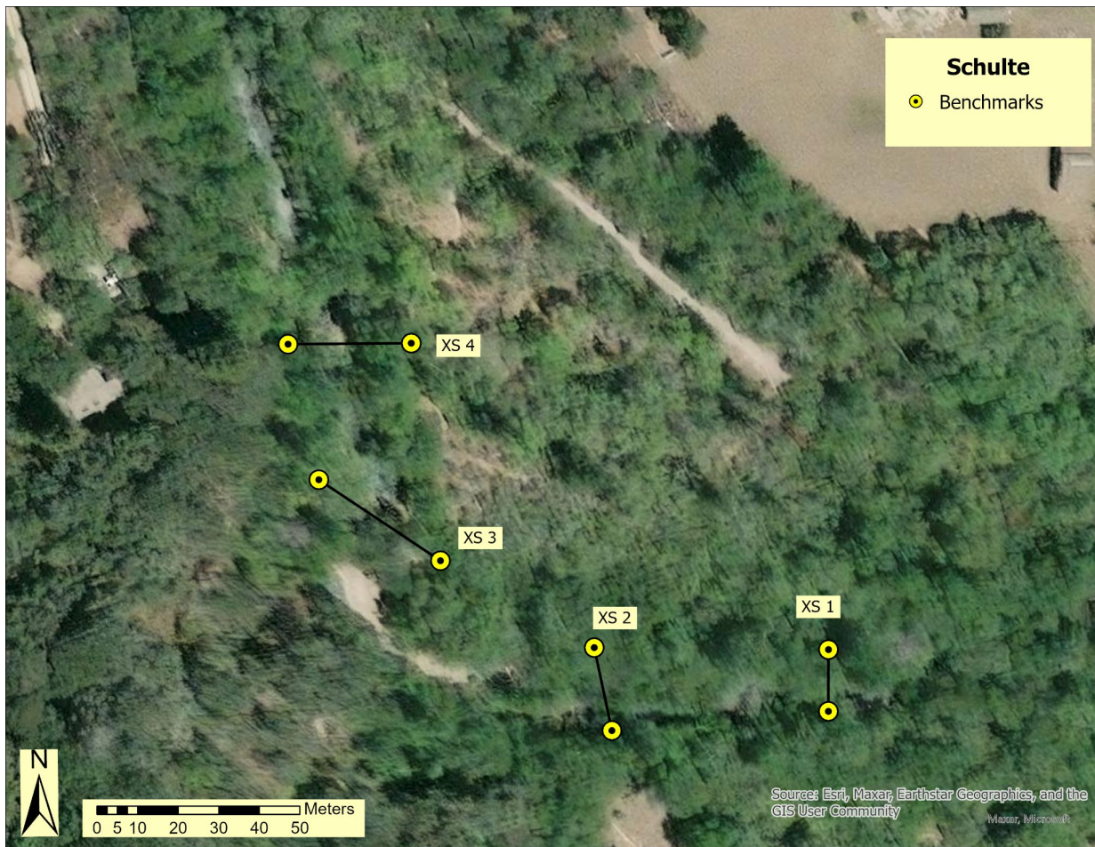
Figure 31. Map of cross sections in SR where autolevel surveys and pebble counts were performed in 2023.
