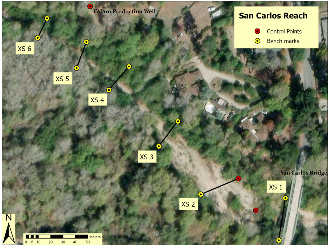
Figure 36: Map of cross sections in SC where autolevel surveys and pebble counts were performed in 2023 (excluding SC 3).
