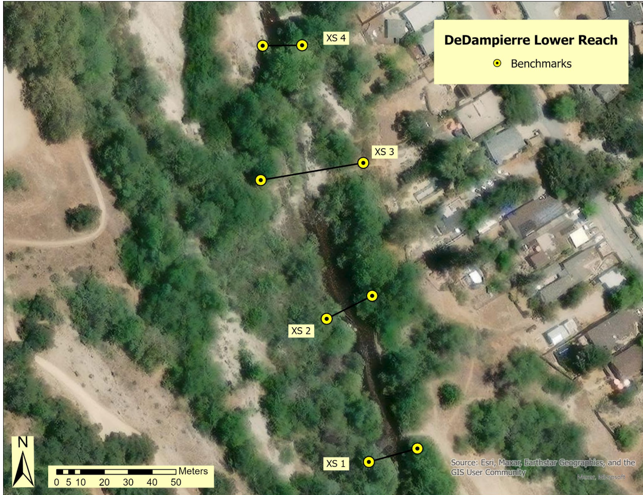
Figure 21. Map of cross sections in DDL where autolevel surveys and pebble counts were performed in 2023.
