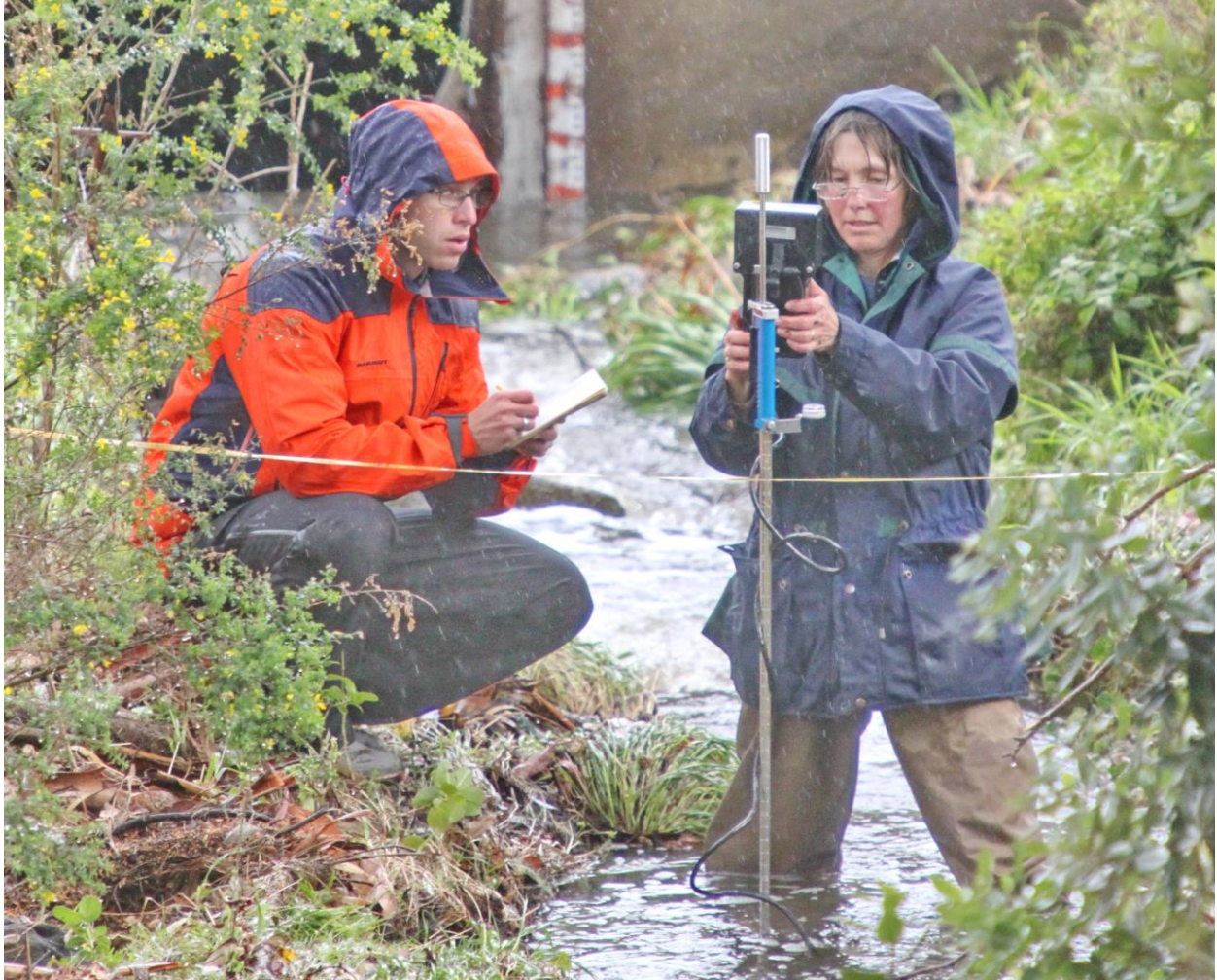
Manual discharge measurement using acoustic Doppler flow velocity meter recordings along cross-section across stream
