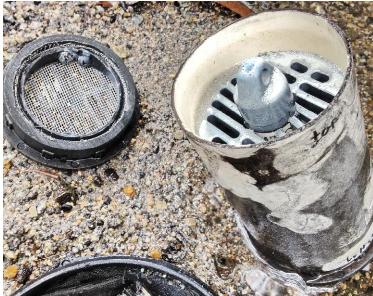
Pressure sensor & built-in logger visible inside inner casing during temporary removal for download.
