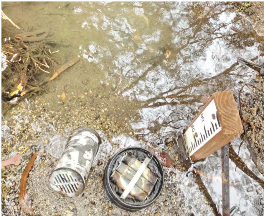
Pressure sensor installed at upper end of Greenwood Park, adjacent to staff plate (outer housing barely visible under water surface; inner housing shown while being removed for download; cap of outer housing also visible)
