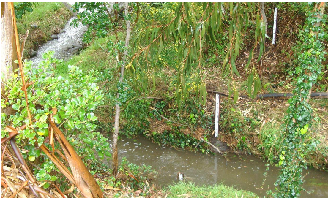
Set of three staff plates installed at upper end of Greenwood Park
