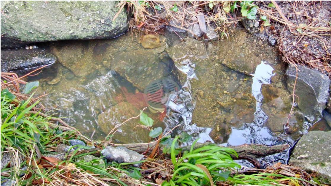
Pressure sensor installed at lower end of Greenwood Park (sensor is beneath grating visible under water surface)
