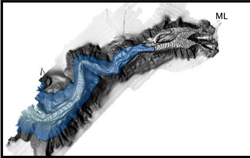
Figure 9: Digital elevation model of low sea level (blue) in Monterey Canyon head. View extends from Moss Landing Harbor (ML) out to sea 4 km, to a depth of 270 m. The rectangular box around “ML” in Figure 2 shows the position of this view. Bathymetric data from the CSUMB Seafloor Mapping Lab ( http://seafloor.csumb.edu/index ).
