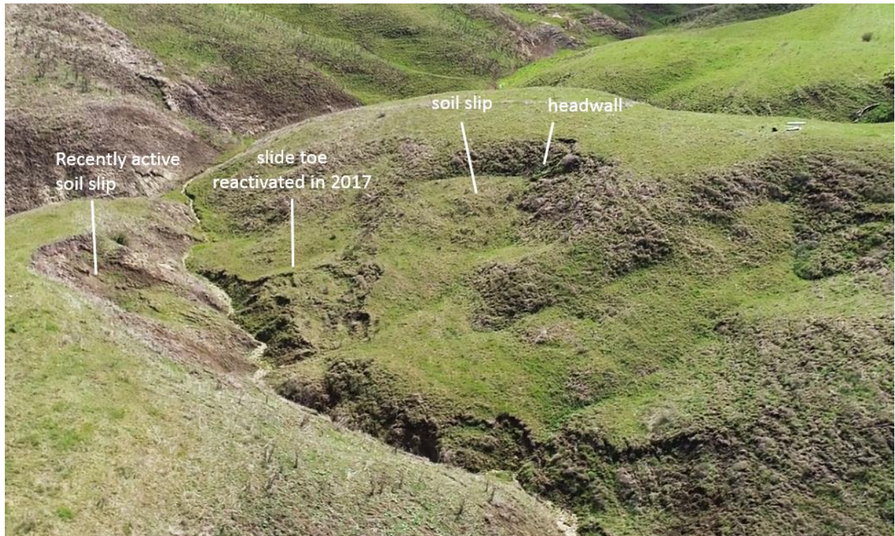
Figure 29. Down gradient view showing unstable slopes in gully system below culvert labeled “2” in Figure 22. Image is oblique aerial view from sUAS. Scene depicts feature five in Figure 22.
