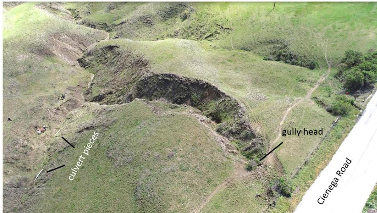
Figure 24. Oblique aerial photograph from sUAS showing active gully near Cienega Road. Feature is labeled “4” in Figure 22. Hillshade of feature is Figure 25. Ground-based photo is Figure 26.
