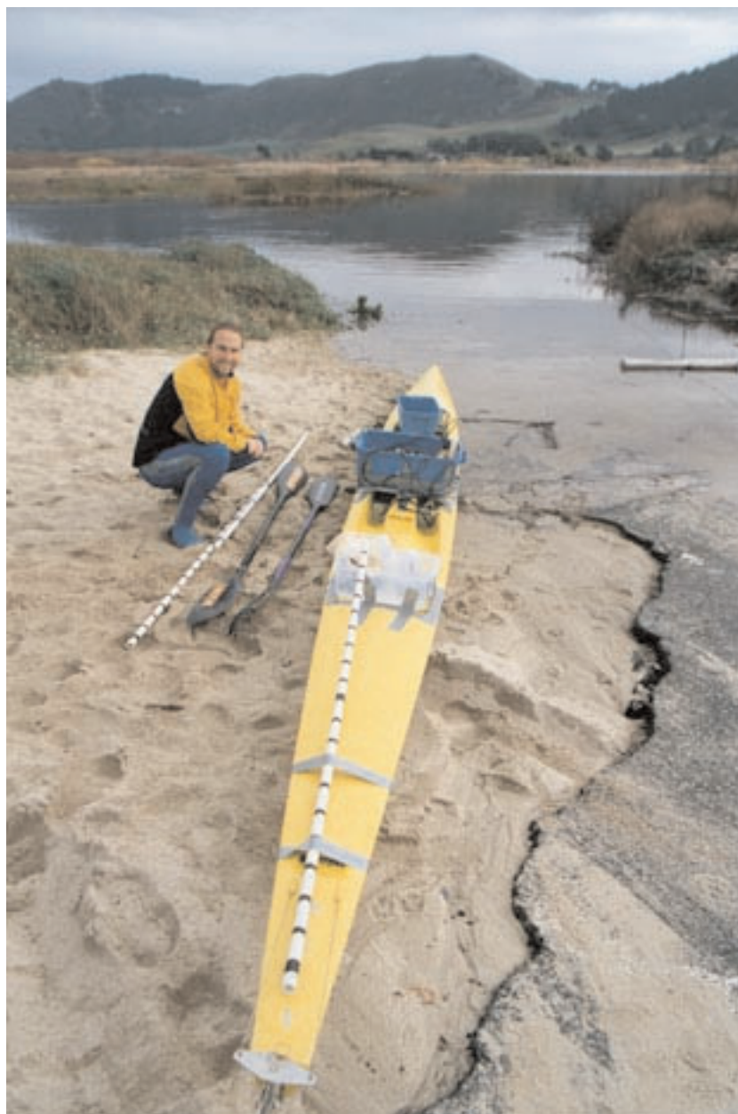
Figure 3.1 One of two tandem kayaks used for water quality monitoring showing the variety of equipment used for collecting water quality information, depth, and bathymetrical data.
