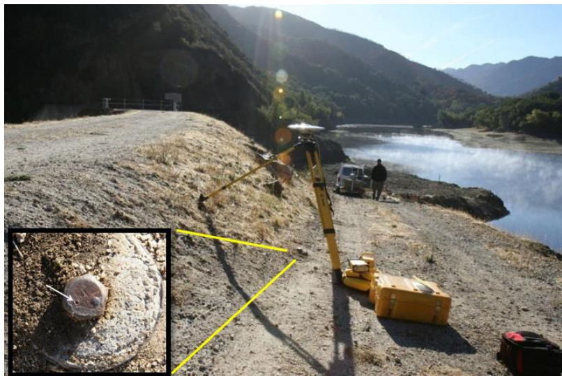
Figure 6: General location of SFML benchmark near the dam crest. Inset shows close up of drill hole used as the horizontal and vertical reference. Photo is from 2008 survey.
