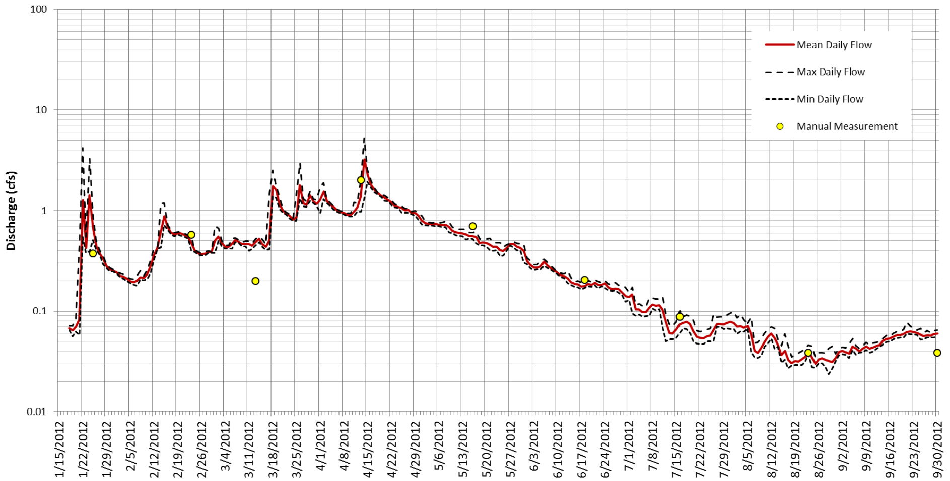
Figure 6. Mean Daily Streamflow at San Clemente Creek gage for Water Year 2012. Red line is mean daily streamflow. Minimum and maximum daily flows are also shown. Yellow points represent manual discharge measurements.
