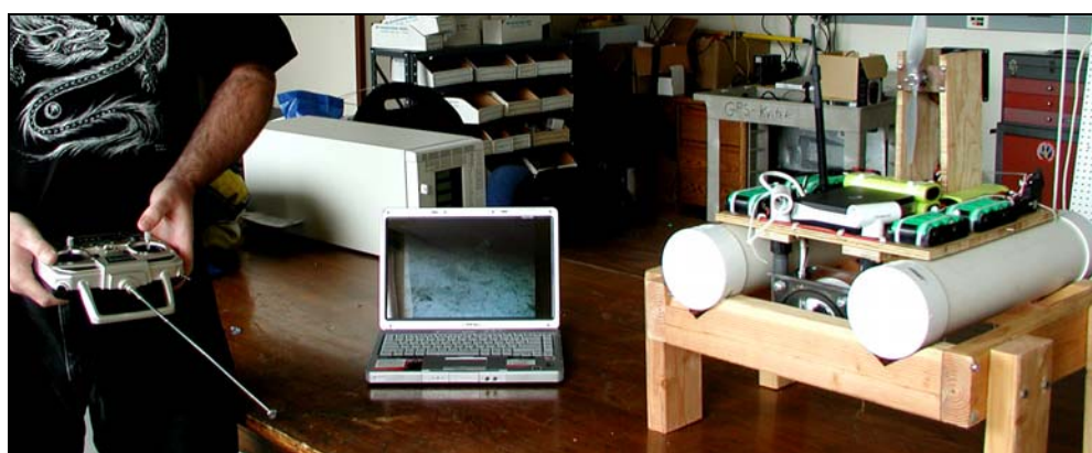
(e) All pieces of the surveillance system: remote control, laptop, and vessel.
