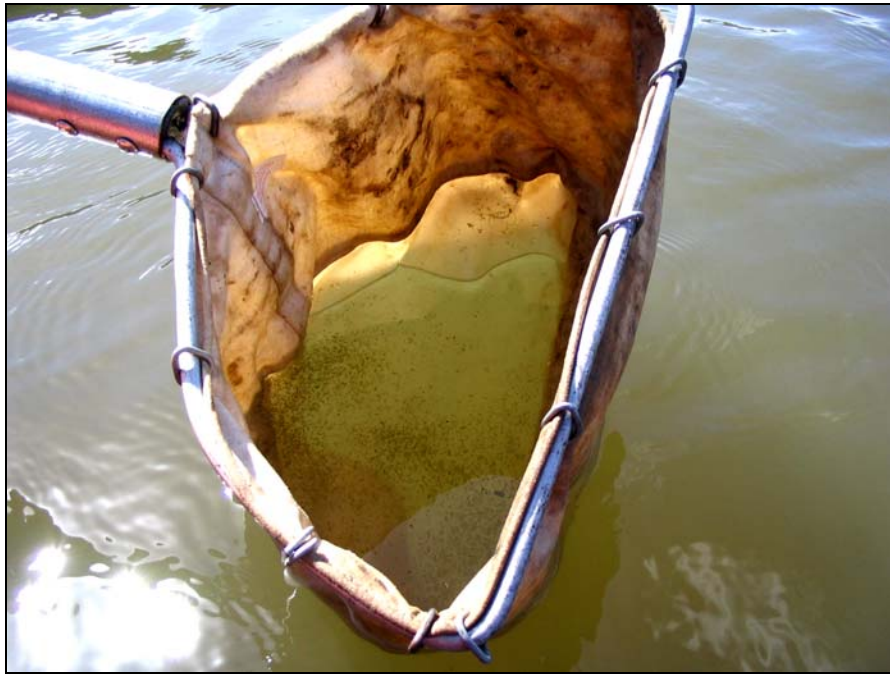
Figure 5-1 D-net used for sampling macroinvertebrates
