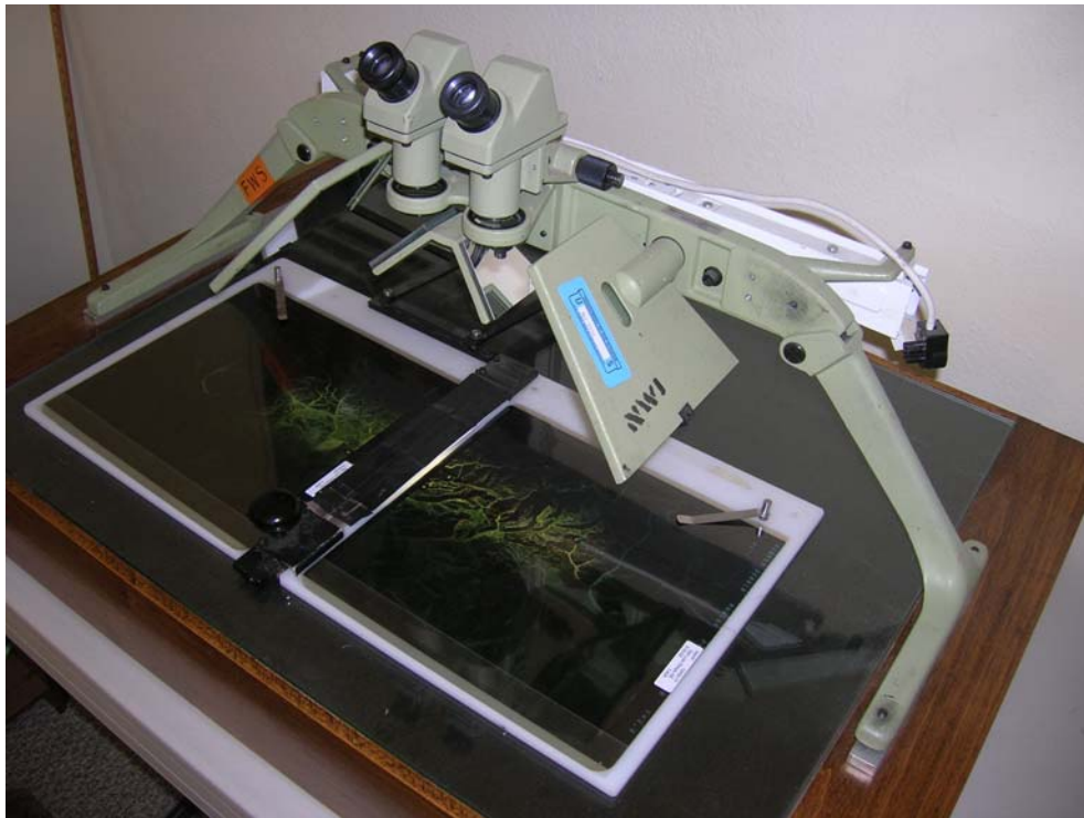
Figure 2. Stereo-scope and light table set used for viewing color inferred stereo photo pairs.
