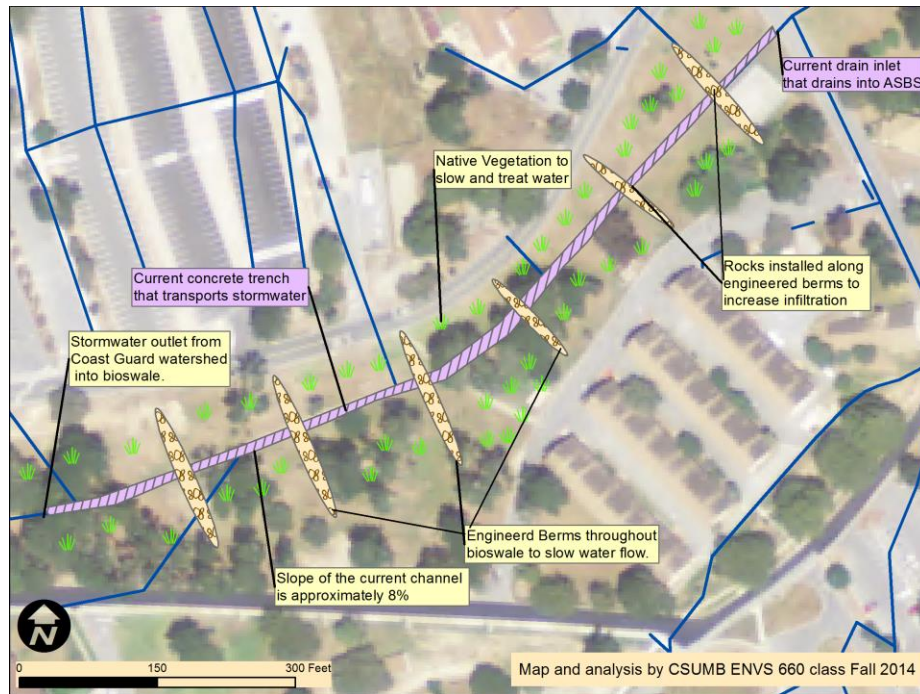
Figure 7: Concept map for bioswale located at LID 4. Bioswale design is illustrated over existing above ground stormwater drainage. Vegetation is represented by green grass.
